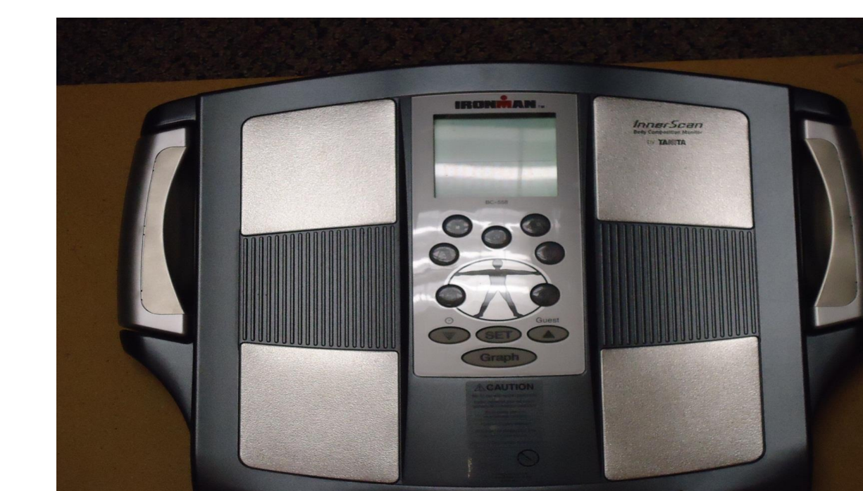
Fig 6. Ironman InnerScan Bioimpedance device to measure standing body composition Parameters (TBW% and FAT%)
