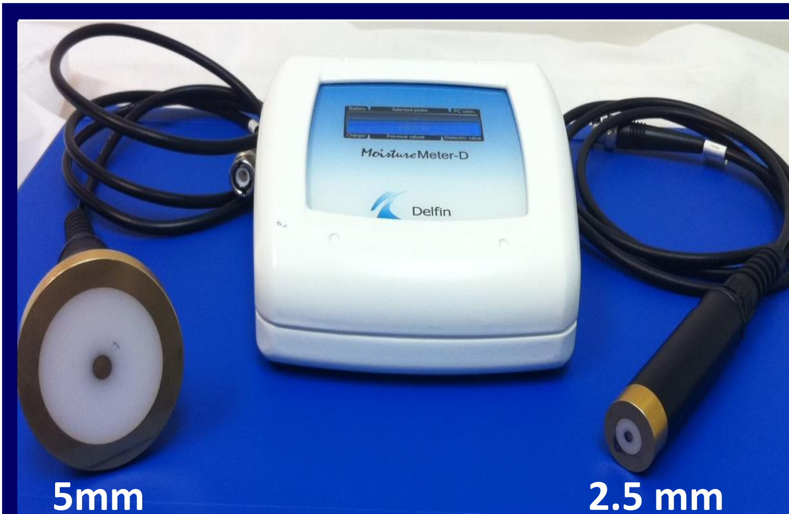
Fig 1. Delfin MoistureMeter-D Control unit with 5.0 and 1.5 mm effective depth probes used in this study
