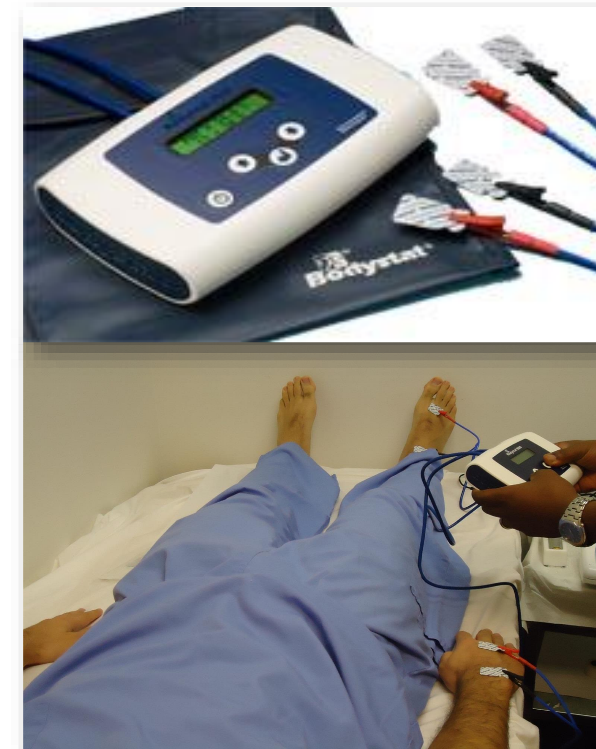
Fig 5. Bodystat bioimpedance device for supine body composition Measurements (TBW% and FAT%)
