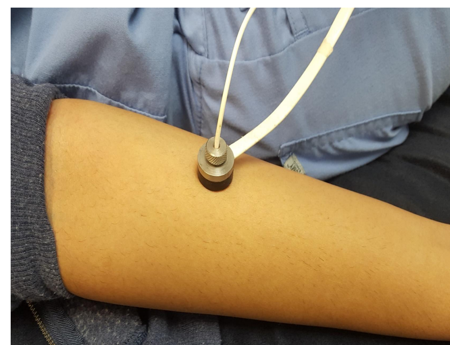
Figure 4: Heating device with laser Doppler probe applied to measurement site.
