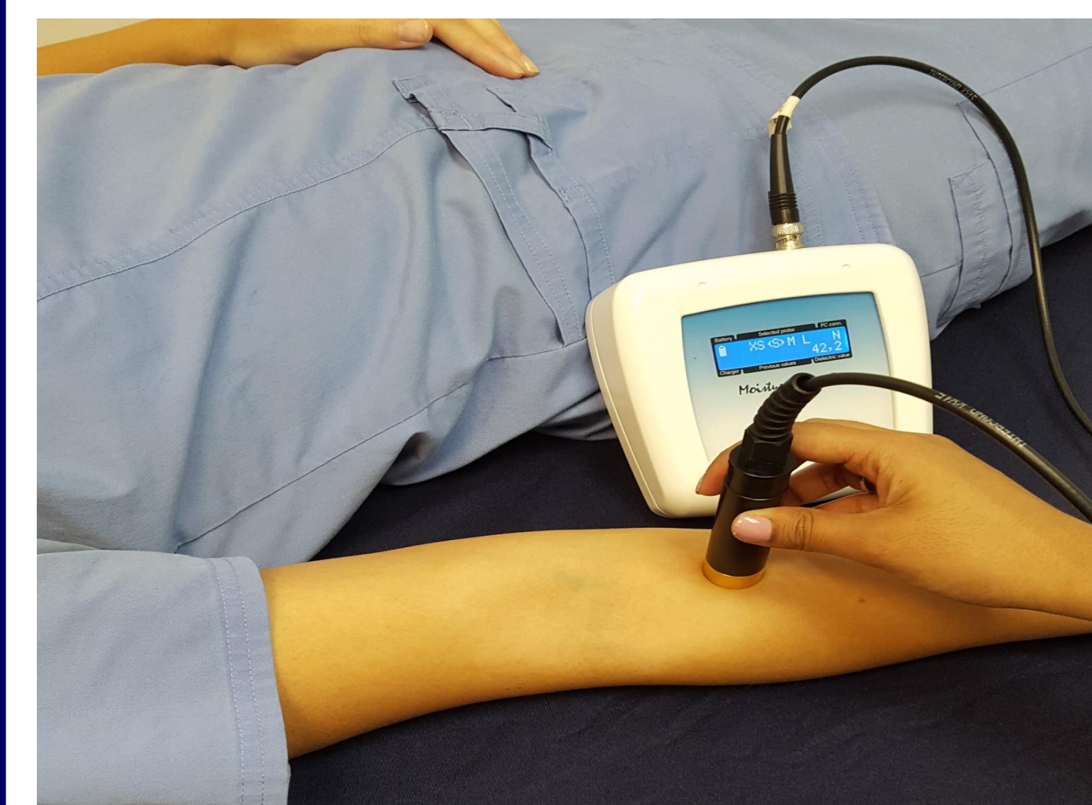
Figure 3: Tissue Dielectric Constant Measurement (TDC using 1.5 and 2.5 mm probes).
