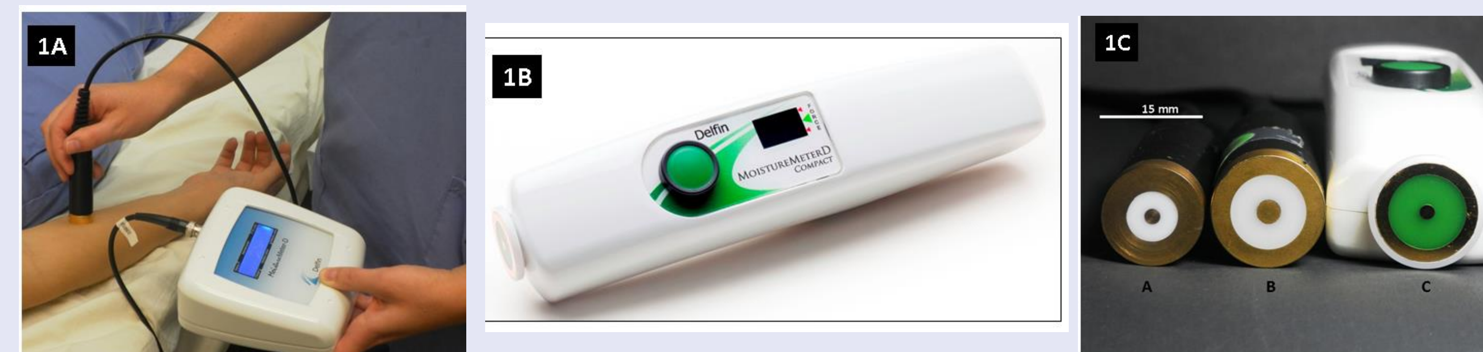
Figure 1: Measurement devices and probes. 1A) MMD unit with probe in contact with forearm skin; 1B) Compact MMDC unit; 1C) Probes shown from measuring surface end. Probes A and B are used with the MMD unit and have effective measurement depths of 1.5 mm for A and 2.5 mm for probe B. Probe C is the self contained MMDC unit.
