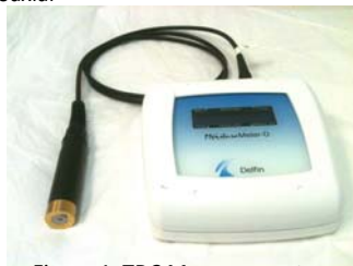
Figure 1. TDC Measurement device and 1.5 mm depth probe.
