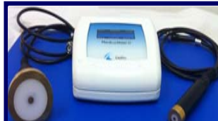
Fig 1: From left to right, 5.0 mm-depth probe, MoistureMeter- D, and 1.5mm-depth probe
